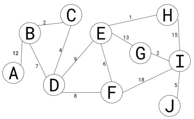
Our task is to get from A to J in the shortest amount of time. The first step is to set up a table containing all the vertices.
