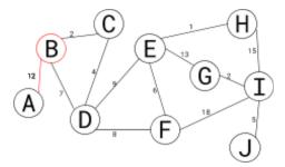
Starting from A, we list all the connections to other nodes. Where A is not connected to the node, we write ∞ because there is effectively no way to get to them - it would take an infinite time to reach them.
