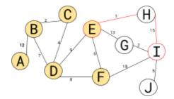
The smallest value in one of the blue columns is 28, column H. H will be the next node to be explored. The shortest path from A has already been found for nodes A B C D E F and H.
