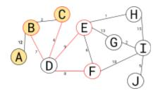
Now, the smallest number in the table in an unexplored column is 18. D is next to be explored. D has no connections to G H I or J, so the time to reach them remains infinite. A B and C have been fully explored so they already have a minimum time. The weight from D to D is 0, so 18 (18 + 0) stays.
