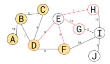
The unexplored nodes are E, G, H, I and J. Out of those, E has the smallest value at 27, so E is next explored. Nodes A B C D F and E already have their shortest paths. The only node which remains unconnected is J, so the weight to it remains infinite.
